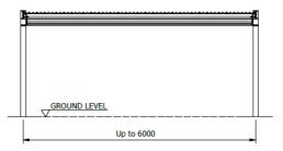
Front profile - Multiple span length
